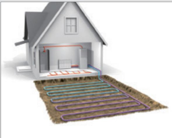
The horizontal ground loop collects solar energy stored in the ground, near the surface. If the bedrock is too deep down, or if you don't want to drill for other reasons, this is a good option.
