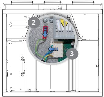
6. Pull the cable bushing at the side of the rotor out as well.
