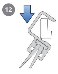
13. Then screw the steel profile back on. Press the sealing strip towards the short end of the steel profile to form a seal. The profile also has a sealing strip along one side. NB: It is important to screw the profile on the right way so that the seal sits tightly against the partition inside the unit. Push the rotor back in.
